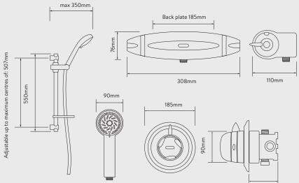
Distance from back face of valve to finished wall surface (includes 10mm allowance for tiles) MIN 60mm, MAX 100mm
