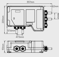
SMARTVALVE - GRAVITY PUMPED
