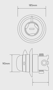
Distance from back face of valve to finished wall surface (includes 10mm allowance for tiles) Min 60mm, Max 100mm
