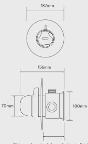
Distance from back face of valve to finished wall surface (includes 10mm allaowance for tiles) Min 68mm, Max 82mm
